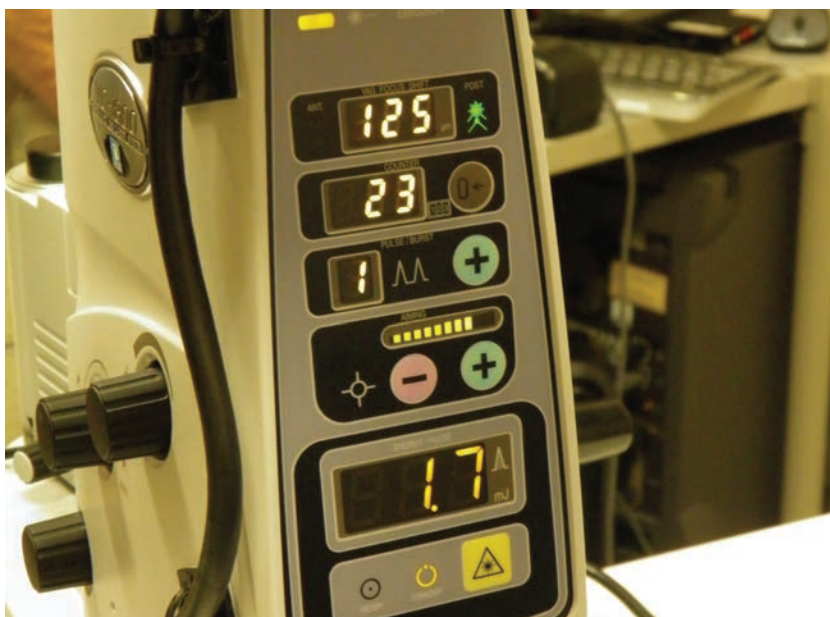
The Nd:YAG laser in action. This particular laser's settings display an offset of 125 \mu m, a total number of 23 laser pulses used in the current procedure, a single pulse (1) per press of the button, and a power level of 1.7mJ.
