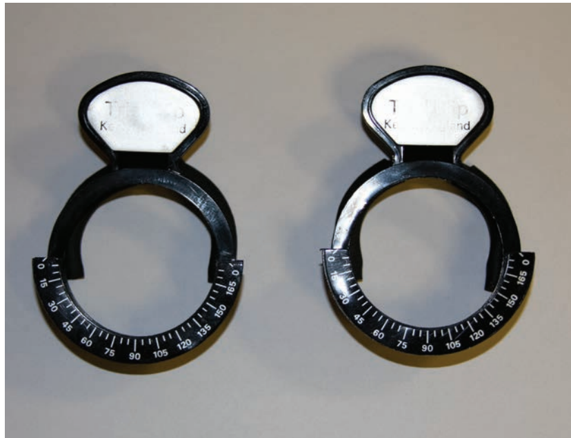
Halberg clips offer convenient demonstration of prescription options by holding the desired trial lenses in place.
