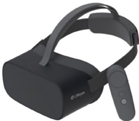
Olleyes virtual reality visual field unit. Full glaucoma threshold visual field capability is available on the device.
