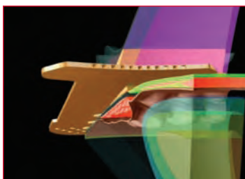
Figure 5. Schematic representation of SOLX Gold Shunt. (Courtesy of SOLX Inc, Waltham, MA)
