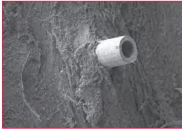
Figure 4. Scanning electron microscopy of iStent trabecular micro bypass stent. (Courtesy of Glaukos Corp, Laguna Hills, CA)
